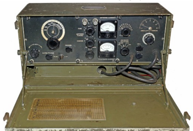
Transmitter-receiver BC-474-A, part of SCR-288-A, resembling the RT-46/TRC-10.
