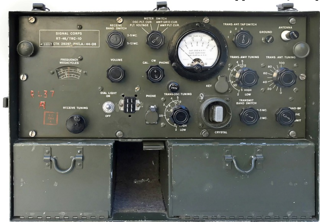
RT-46/TRC-10. Note that the 6-pin power plug was not original and substituted later. The crystal cover was missing.
